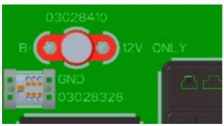
Add an additional 4ga. battery cable from the B+ Whelen stud to the red stud in the top right cornet of the junction box.
