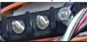
Part number 0311787 HARNESS RH TOOLBOX WIRING 2012 is brought across the subframe and into the toolbox through the larger opening at the top. Connect it to the mating connector hanging off of the junction box.
